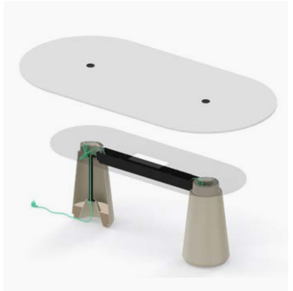
Integrated electrical management consisting of an electrified column and an electrification trunking connecting the two columns. One of the two columns is electrified with an inner tube made of steel with a diameter of 40 mm and bolted to the bottom of the column. The electrification tray is made of folded sheet steel with a thickness of 3 mm.
