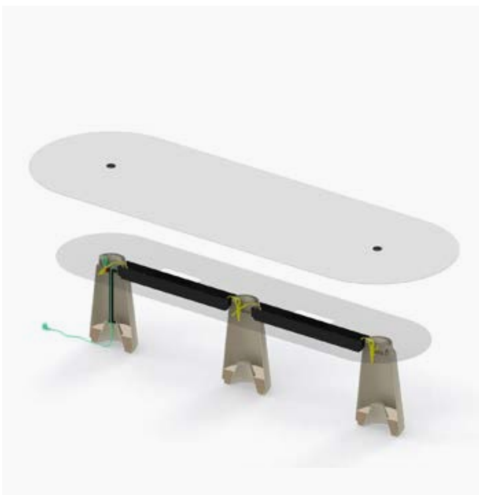
Integrated electrical management consisting of an electrified column and a two cables tray connecting the three columns. One of the three columns is electrified with an inner tube made of steel with a diameter of 40 mm and bolted to the bottom of the column. The electrification tray is made of folded sheet steel with a thickness of 3 mm.
